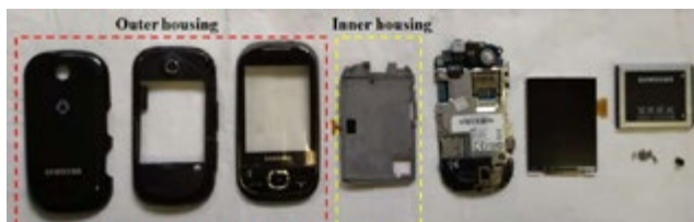
Figure 2: Outer housing parts (in red) with an inner housing part (yellow). Source: Authors.
