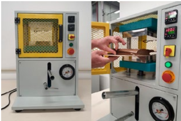
Figure 02: Hydraulic Press for Crushing with Heating. Source: Authors.
